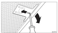
If a grease filter is inadvertently refitted upside down, insert a small screwdriver blade into the slit to disengage the clip.
