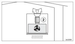
The silencer needs to be positioned between the exhaust connection and the exhaust grille ②. Ensure there is adequate space for fitting it.
