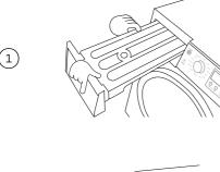
Remove the water tank by holding onto the handle and pulling outwards gently. Ensure the tank is kept level when removed to prevent the water from spilling.
