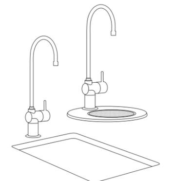
Filter Tap can be installed over sink or optional font
