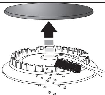
Check the burner slots are not blocked. If a blockage occurs, remove stubborn particles using a toothbrush (**Fig. 6.4**).
