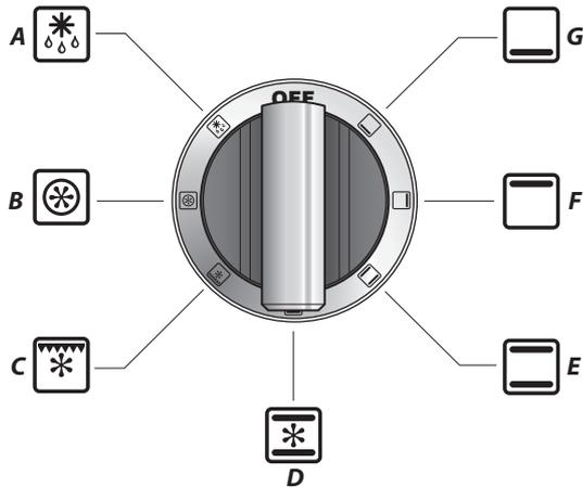
A – Defrost, B – Fan oven, C – Fanned grilling, D – Fan assisted oven, E – Conventional oven, F – Browning element, G – Base heat
